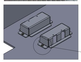
STEP 2: ALIGN UNIT IN POSITION THEN REMOVE THE CABINET AND USE 1/4" SELF-TAPPING SCREWS AND WASHERS TO FASTEN FEET TO THE FLOOR.
