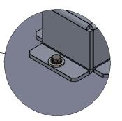
STEP 3: REATTACH THE CABINET USING 14-20 BOLTS AND **NYLOC NUTS**
