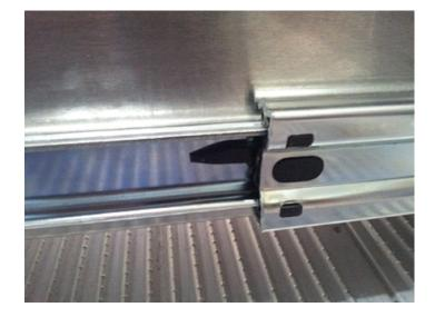
STEP 1: REMOVE DRAWERS USING TABS ON SLIDES
