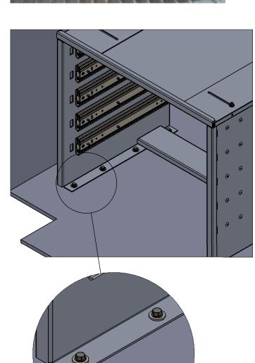
ALIGN UNIT IN POSITION AND USE 1/4" SELF-TAPPING SCREWS AND WASHERS TO FASTEN CABINET TO THE FLOOR THROUGH THE HOLES IN THE BOTTOM FLANGE OF THE SIDE PANELS.
