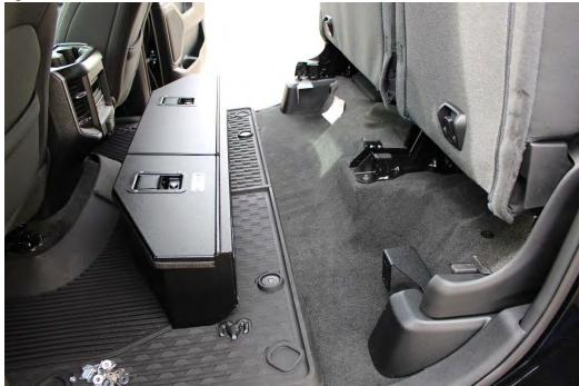
4. Position the box at the back, touching the Install brackets.
