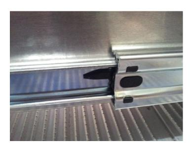
STEP 1: REMOVE DRAWERS USING TABS ON SLIDES
